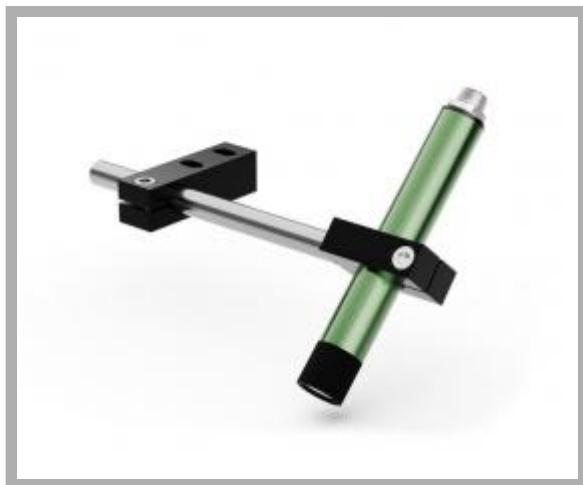
**Type of projection:** Dot**Supply voltage:** 9-36 Vdc 10-30 Vac**Connection:** M12 connector + cm 500 cable**Light source:** Laser diode**Casing:** Green anod.alum.**Dimension:** 20x145 mm**Protection class:** IP67**Storage temperature °C/°F:** -40 +85 °C / -40 +185 °F**Operating temperature °C/°F:** -20 +60 °C / -4 +140 °F
