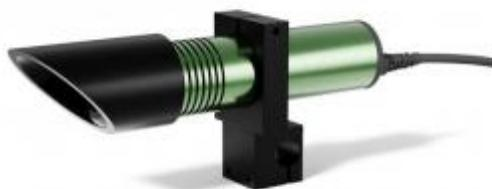
**Type of projection:** Line**Supply voltage:** 80-265 Vac**Connection:** Cable 3x0,75 cm 300 without plug**Light source:** Laser diode**Casing:** Green anod.alum.**Dimension:** 50X220 mm**Protection class:** IP67**Storage temperature °C/°F:** -40 +85 °C / -40 +185 °F**Operating temperature °C/°F:** -20 +60 °C / -4 +140 °F
