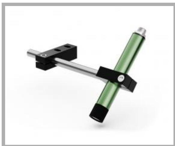
**Type of projection:** Cross**Supply voltage:** 9-36 Vdc 10-30 Vac Trigger 5-30Vdc**Connection:** M12 connector + cm 500 cable**Light source:** Laser diode**Casing:** Green anod.alum.**Dimension:** 20x145 mm**Protection class:** IP67**Storage temperature °C/°F:** -40 +85 °C / -40 +185 °F**Operating temperature °C/°F:** -20 +60 °C / -4 +140 °F
