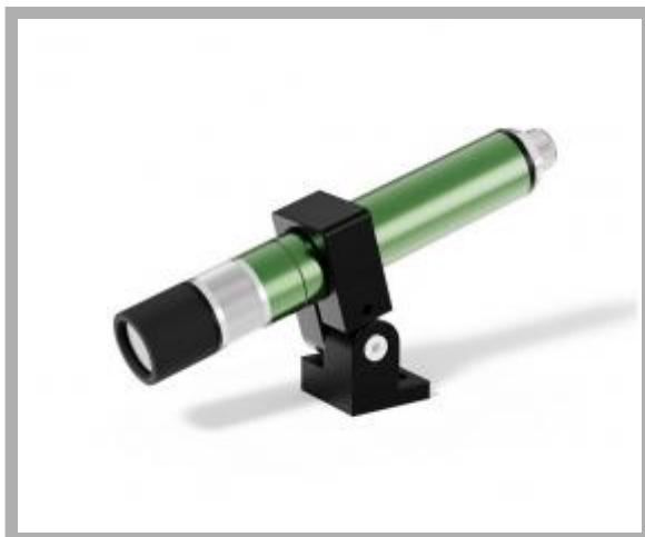
**Type of projection:** Dot**Supply voltage:** 9-36 Vdc 10-30 Vac Trigger 5-30Vdc**Connection:** M12 connector + cm 500 cable**Light source:** Laser diode**Casing:** Green anod.alum.**Dimension:** 20x135 mm**Protection class:** IP67**Storage temperature °C/°F:** -40 +85 °C / -40 +185 °F**Operating temperature °C/°F:** -20 +60 °C / -4 +140 °F
