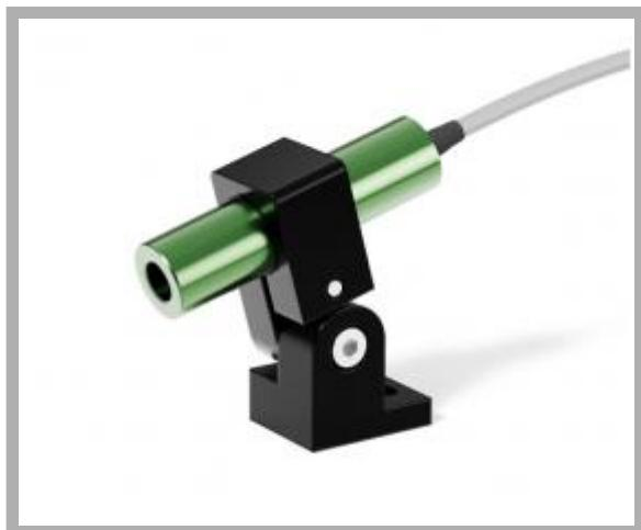
**Type of projection:** Dot**Supply voltage:** 5 Vdc**Connection:** Cable 2x0,25 cm 200**Light source:** Laser diode**Casing:** Green anod.alum.**Dimension:** 14x55 mm**Protection class:** IP64**Storage temperature °C/°F:** -40 +85 °C / -40 +185 °F**Operating temperature °C/°F:** -10 +50 °C / 14 +122 °F
