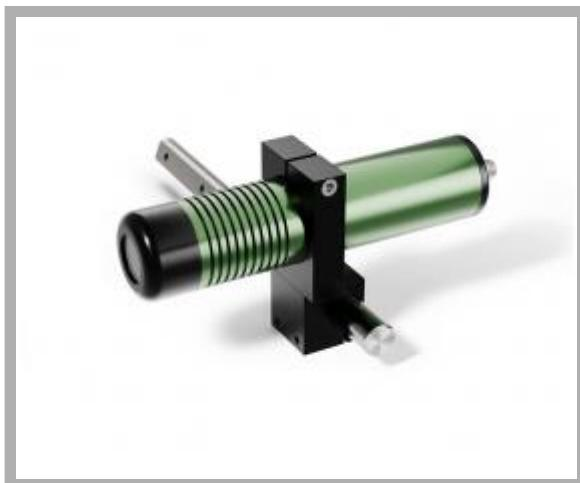
**Type of projection:** Line**Supply voltage:** 9-36 Vdc 10-30 Vac**Connection:** M12 connector + cm 500 cable**Light source:** Laser diode**Casing:** Green anod.alum.**Dimension:** 50X230 mm**Protection class:** IP67**Storage temperature °C/°F:** -40 +85 °C / -40 +185 °F**Operating temperature °C/°F:** -10 +50 °C / 14 +122 °F
