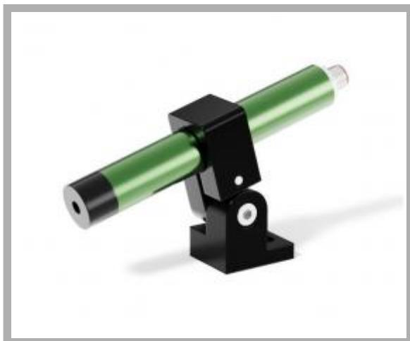
**Type of projection:** Cross**Supply voltage:** 5-30 Vdc**Connection:** M8 connector + cm 300 cable**Light source:** Laser diode**Casing:** Green anod.alum.**Dimension:** 14x95 mm**Protection class:** IP64**Storage temperature °C/°F:** -40 +85 °C / -40 +185 °F**Operating temperature °C/°F:** -10 +50 °C / 14 +122 °F
