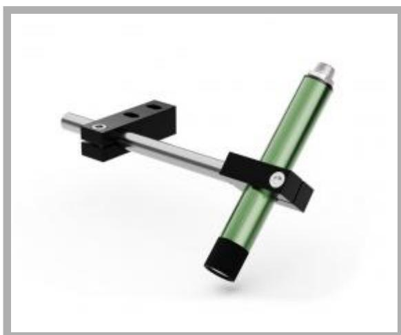
**Type of projection:** Circle**Supply voltage:** 9-36 Vdc 10-30 Vac**Connection:** M12 connector + cm 500 cable**Light source:** Laser diode**Casing:** Green anod.alum.**Dimension:** 20x145 mm**Protection class:** IP67**Storage temperature °C/°F:** -40 +85 °C / -40 +185 °F**Operating temperature °C/°F:** -20 +60 °C / -4 +140 °F
