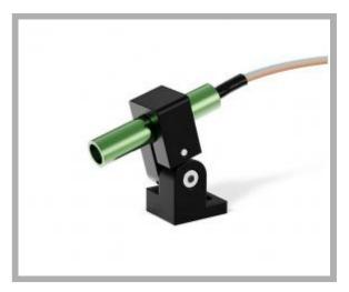
Type of projection: Dot Supply voltage: 5 Vdc Connection: Blue/brown wires cm 30 Light source: Laser diode Casing: Green anod.alum. Dimension: 11X55 mm Protection class: IP64 Storage temperature °C/°F: -40 +85 °C / -40 +185 °F Operating temperature °C/°F: -10 +50 °C / 14 +122 °F
