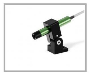
Type of projection: Line Supply voltage: 5-30 Vdc Connection: Cable 2x0,25 cm 200 Light source: Laser diode Casing: Green anod.alum. Dimension: 11X65 mm Protection class: IP64 Storage temperature °C/°F: -40 +85 °C / -40 +185 °F Operating temperature °C/°F: -10 +50 °C / 14 +122 °F
