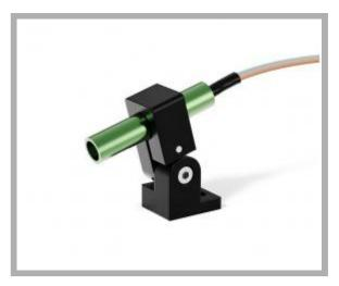
Type of projection: Dot Supply voltage: 5-30 Vdc Connection: Blue/brown wires cm 30 Light source: Laser diode Casing: Green anod.alum. Dimension: 11X55 mm Protection class: IP64 Storage temperature °C/°F: -40 +85 °C / -40 +185 °F Operating temperature °C/°F: -10 +50 °C / 14 +122 °F
