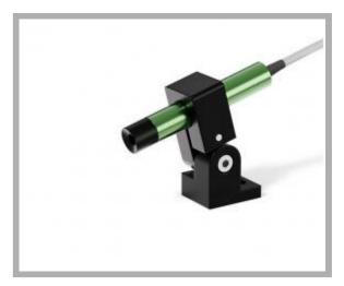
Type of projection: Line Supply voltage: 5 Vdc Connection: Cable 2x0,25 cm 200 Light source: Laser diode Casing: Green anod.alum. Dimension: 11X65 mm Protection class: IP64 Storage temperature °C/°F: -40 +85 °C / -40 +185 °F Operating temperature °C/°F: -10 +50 °C / 14 +122 °F
