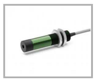
Type of projection: Cross Supply voltage: 5 Vdc Connection: Cable 2x0,25 cm 200 Light source: Laser diode Casing: Green anod.alum. Dimension: 14x65 mm Protection class: IP64 Storage temperature °C/°F: -40 +85 °C / -40 +185 °F Operating temperature °C/°F: -10 +50 °C / 14 +122 °F
