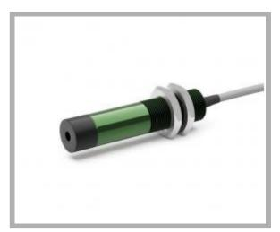
Type of projection: Line Supply voltage: 5 Vdc Connection: Cable 2x0,25 cm 200 Light source: Laser diode Casing: Green anod.alum. Dimension: 14x65 mm Protection class: IP64 Storage temperature °C/°F: -40 +85 °C / -40 +185 °F Operating temperature °C/°F: -10 +50 °C / 14 +122 °F
