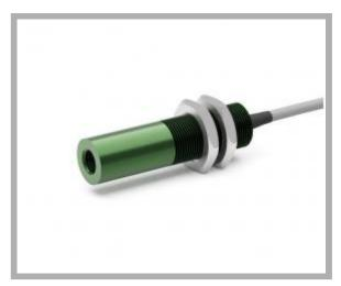
Type of projection: Dot Supply voltage: 5-30 Vdc Connection: Cable 2x0,25 cm 200 Light source: Laser diode Casing: Green anod.alum. Dimension: 14x55 mm Protection class: IP64 Storage temperature °C/°F: -40 +85 °C / -40 +185 °F Operating temperature °C/°F: -10 +50 °C / 14 +122 °F
