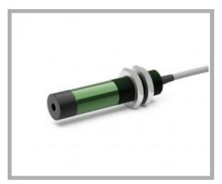
Type of projection: Circle Supply voltage: 5-30 Vdc Connection: Cable 2x0,25 cm 200 Light source: Laser diode Casing: Green anod.alum. Dimension: 14x65 mm Protection class: IP64 Storage temperature °C/°F: -40 +85 °C / -40 +185 °F Operating temperature °C/°F: -10 +50 °C / 14 +122 °F
