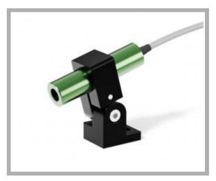
Type of projection: Dot Supply voltage: 5 Vdc Connection: Cable 2x0,25 cm 200 Light source: Laser diode Casing: Green anod.alum. Dimension: 14x55 mm Protection class: IP64 Storage temperature °C/°F: -40 +85 °C / -40 +185 °F Operating temperature °C/°F: -10 +50 °C / 14 +122 °F
