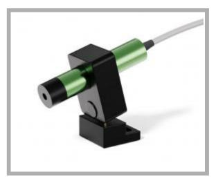
Type of projection: Circle Supply voltage: 5 Vdc Connection: Cable 2x0,25 cm 200 Light source: Laser diode Casing: Green anod.alum. Dimension: 14x65 mm Protection class: IP64 Storage temperature °C/°F: -40 +85 °C / -40 +185 °F Operating temperature °C/°F: -10 +50 °C / 14 +122 °F
